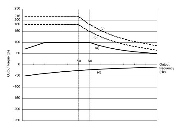
Figure 3.2 Output Torque Characteristics (Base frequency: 60 Hz)
