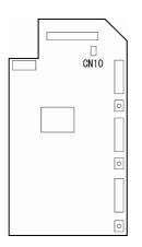
Figure 8.5 Location of USB Connector on Control PCB
