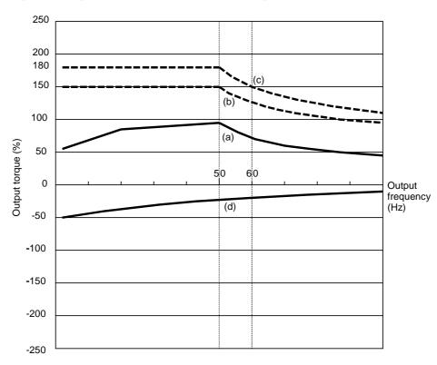
Figure 3.1 Output Torque Characteristics (Base frequency: 50 Hz)
