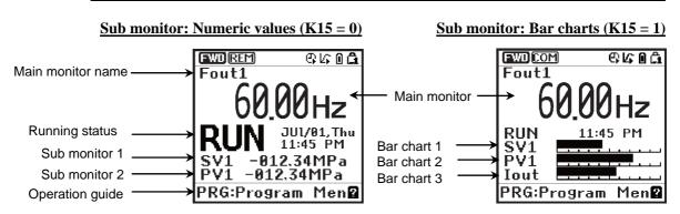
The display type can be selected easily in Programming mode as follows. PRG > 1(Start-up) > 4(Disp Setting) > 1(Disp Mode)
