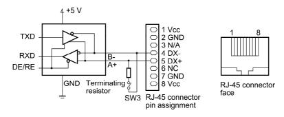
Note Pins 1, 2, 7, and 8 on the RJ-45 connector are exclusively assigned to power supply and grounding for keypads. When connecting other devices to the RJ-45 connector, take care not to use those pins. Failure to do so may cause a short-circuit hazard. Use pins 4 and 5 only.
