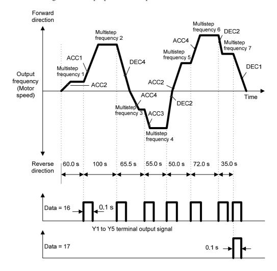
To start or stop a pattern operation, use the  $\mathbb{E}_{O}$  keys on the keypad or turn the related input terminals ON/OFF.
