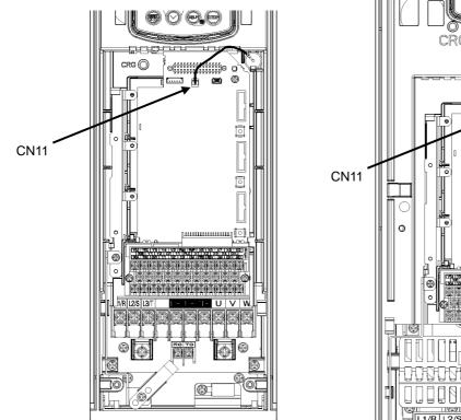
Figure 4.14 Battery Loaded (200 V class series inverters of 3.7 kW or below and 400 V ones of 7.5 kW or below)
