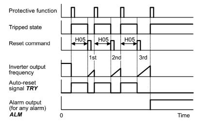
The auto-reset operation can be monitored from the external equipment by assigning the digital output signal *TRY* to any of the programmable, output terminals [Y1] to [Y4], [Y5A/C], and [30A/B/C] with any of E20 through E24 and E27 (data = 26).
