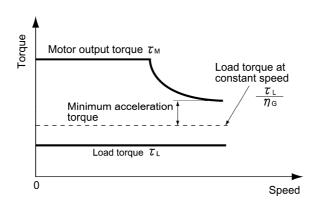
Figure 3.4 Example Study of Minimum Acceleration Torque
