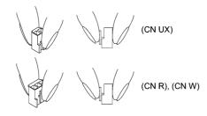
Figure 5.4-4 Removing/Inserting the Jumpers
