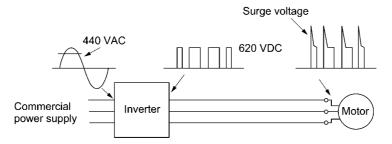
Figure B.1 Voltage Waveform of Individual Portions
