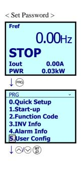
$\underbrace{\stackrel{\text{(ESET)}}{\stackrel{}_{X \rightarrow 0}}} \text{Return to previous screen} \quad (\stackrel{\text{(PRG)}}{\stackrel{}_{X \rightarrow 0}} \text{Return to running mode}$
