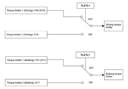
■ Torque limiter for braking (Frequency increment limit) (H76)
