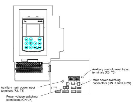
Figure 5.4-3 Location of Switching Connectors (400 V class series inverters of 160 kW or above)
