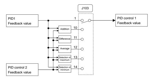
PID control 2 feedback selection block diagram
