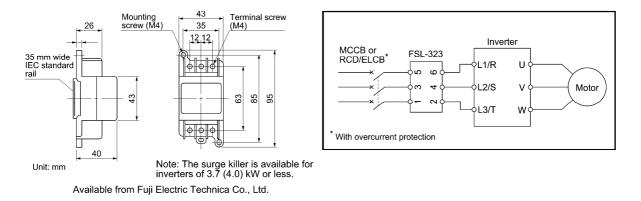
Figure 4.3 Dimensions of Surge Killer and Connection Example
