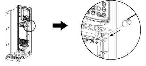
(3) Hook the battery harness over the boss and then fully insert the connector into connector CN11 on the control printed circuit board.
