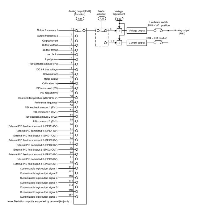
Figure 7.6 Terminal [FM1] Output Selector
