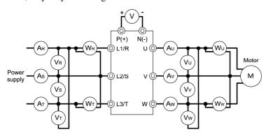
Figure 10.1 Connection of Meters
