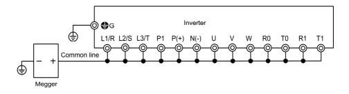
Figure 10.2 Main Circuit Terminal Connection for Megger Test
