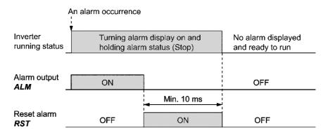
Enable external alarm trip -- THR (Function code data = 9)
