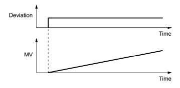
D differential time (External PID control 1: J512, External PID control 2: J612, External PID control 3: J662)
