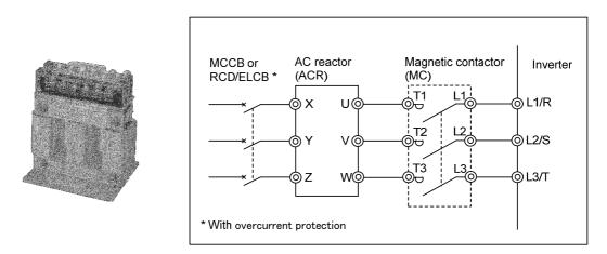
Figure 4.6 External View of AC Reactor (ACR) and Connection Example
