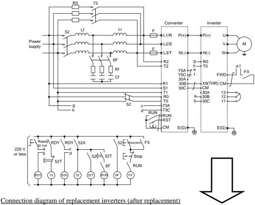
Connection diagram of conventional inverters (before replacement)
