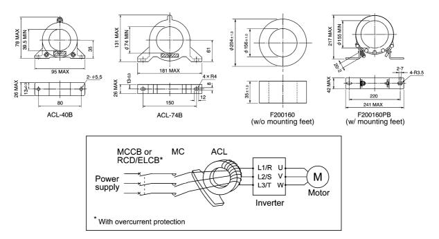
Figure 4.8 Dimensions of Zero-phase Reactor for Reducing Radio Noise (ACL) and Connection Example
