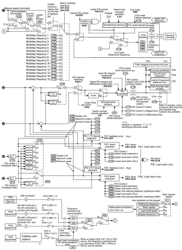
\*1 Priority when the same function is selected by E61 to E63 U87 >···> U81 > Terminal [12] > Terminal [C1] > Terminal [V2] > Terminal [32] > Terminal [C2] > Terminal [PT1] > Terminal [PT2]
