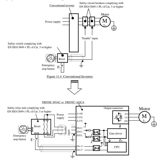
\*Transistor output terminals (e.g., [Y1]-[CMY], DECF (Function code data=1101), Refer to Section 11.1.4.6)
