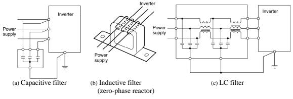
Figure A.10 Various Filters and their Connection
