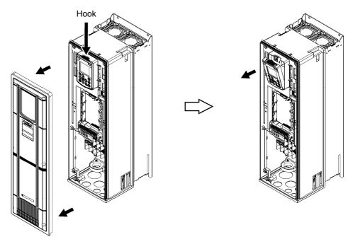
Figure 5.7 Removing the Keypad
