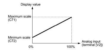
Example: To detect 0 to 30 kPa with 1 to 5 V output of the pressure sensor
