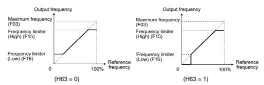
• When you change the frequency limiter (High) (F15) in order to raise the reference frequency, be sure to change the maximum frequency (F03) accordingly.
