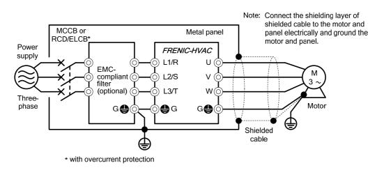
Figure 11.2-1 Mounting the Inverter with EMC-compliant Filter in a Metal Panel
