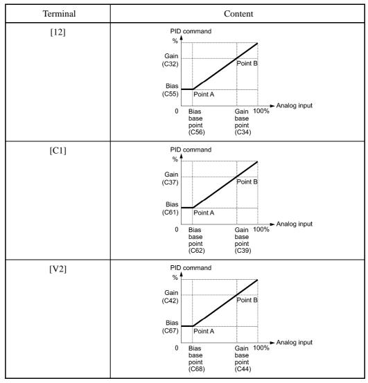
(Example) Mapping the range of 1 through 5 V at terminal [12] to 0 through 100%
