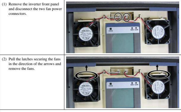
(3) Mount the internal fans in the reverse order of removal.
