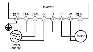
Figure 5.17 Connection of Main Circuit Terminals
