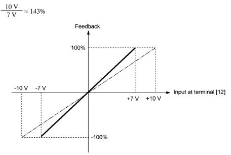
(Example 2) When the output level of the external sensor is 0 to 10 VDC:
