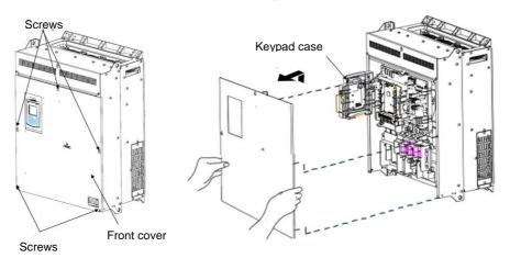
Figure 5.3 Removing the Front Cover and the Wiring Plate (FRN110AR1S-4D)
