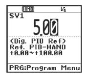
Figure 5.15 Setting the PID Process Command (display sample)
