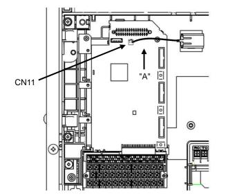
Insert the battery until it is secured by the latch on the battery holder.
