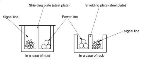
Figure A.7 Separate Wiring
