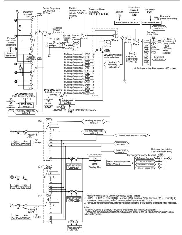
Figure 7.1 (2) Frequency Command Block
