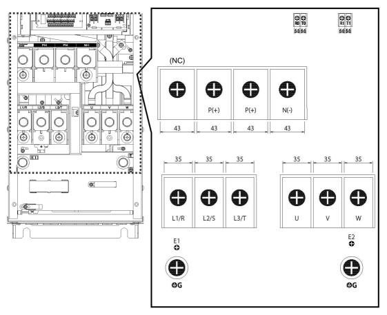
(NC): No connection (Do not make wiring.)
