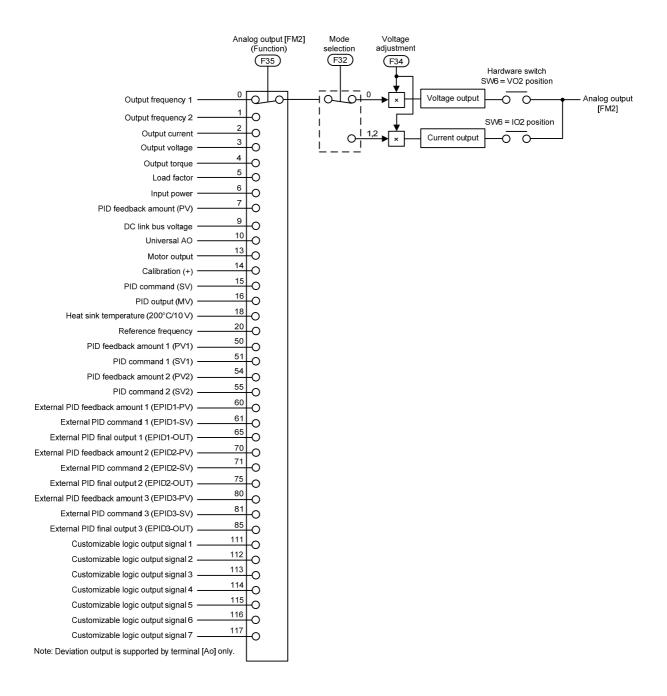
Figure 7.7 Terminal [FM2] Output Selector
