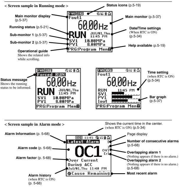
Figure 5.12 Screen Samples In Running and Alarm Modes
