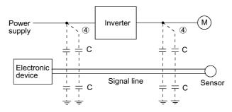
Figure A.5 Electrostatic Induced Noise
