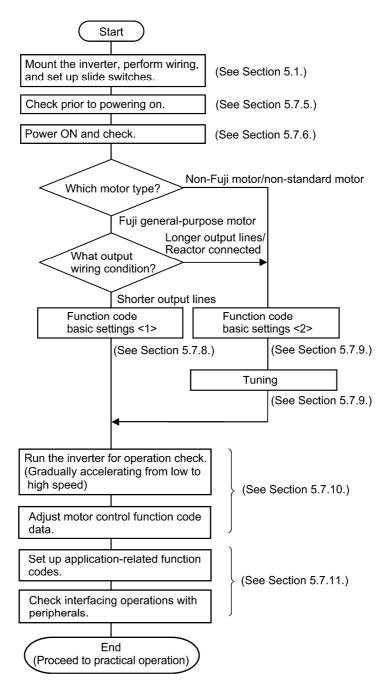
Figure 5.16 Test Run Procedure
