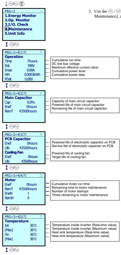
Use the ⊘/ ⊗ keys to select [4. Maintenance], and confirm with the (ﷺ) key.
