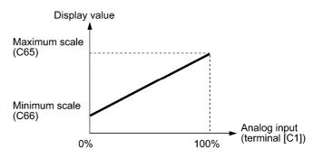
Example: To detect 0 to 30 kPa with 4 to 20 mA output of the pressure sensor
