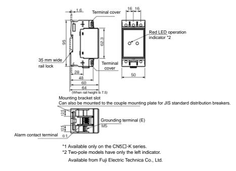
Figure 4.4 Arrester Dimensions and Connection Examples
