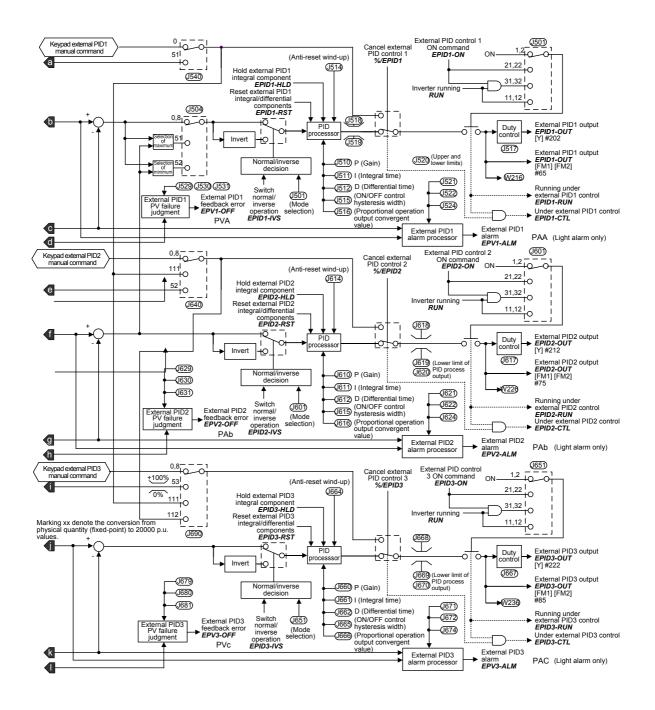
Figure 7.5 (2) External PID Process Control Block
