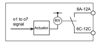
Figure 4.12 Internal Circuits
