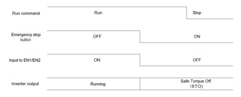
Figure 11.7 Inverter Output State when the Emergency Stop Button is Turned ON with the Inverter Running
