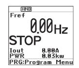
Figure 5.18 Display of the LCD Monitor after Power-on
