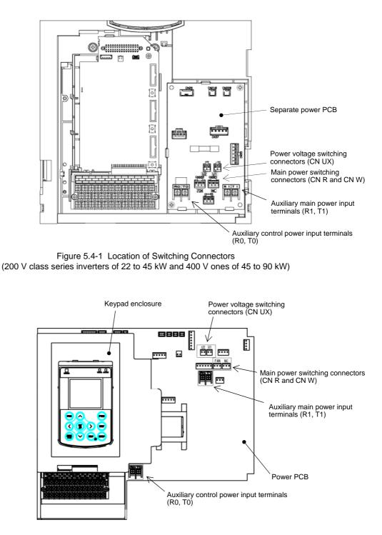
Figure 5.4-2 Location of Switching Connectors (200 V class series inverters of 55 to 90 kW and 400 V ones of 110 to 132 kW)
