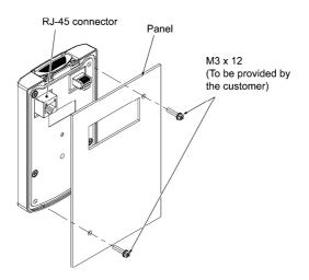
Figure 5.9 Mounting the Keypad
