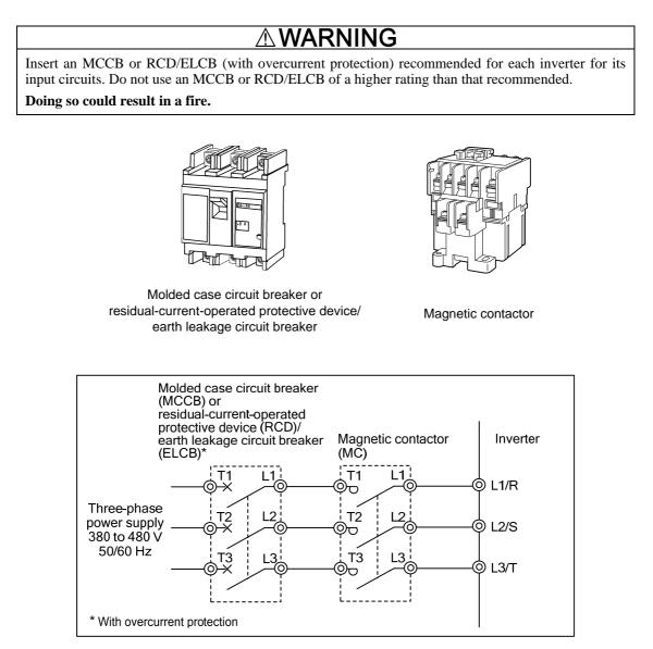
Figure 4.2 External Views of MCCB or RCD/ELCB and MC and Connection Example
