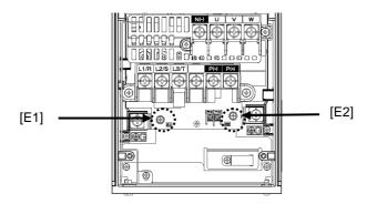
• FRN22AR1■-2□ to FRN45AR1■-2□, FRN45AR1■-4□ to FRN90AR1■-4□ Secure the filter grounding wires to the supports, using the screws removed from terminals [E1] and [E2].
