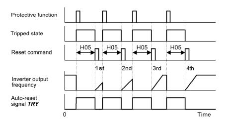
• In the figure below, the inverter fails to restart normal operation within the number of reset times specified by H04 (in this case, 3 times (H04 = 3)), and issues the alarm output (for any alarm) *ALM*.
