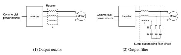
Figure B.3 Method to Suppress Surge Voltage
