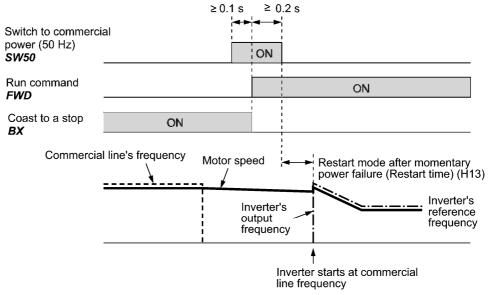
• When the motor speed decreases significantly during coast-to-stop (with the current limiter activated):
