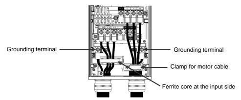
Figure 11.1 Wiring to Main Circuit Terminals
