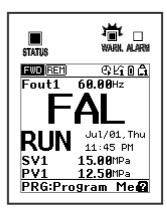
Fig. 9.1 Light alarm display example
