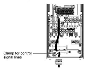
Figure 11.2 Wiring to Control Circuit Terminals
