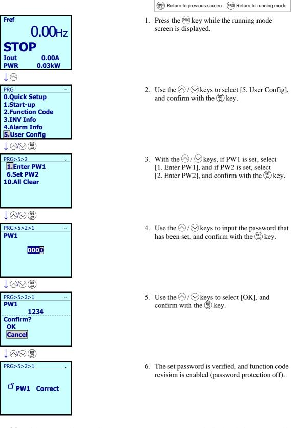
If the password is entered incorrectly, **<u>APW Incorrect</u>** is displayed. If the password is mistaken five times, operations become impossible (alarm sounds).
