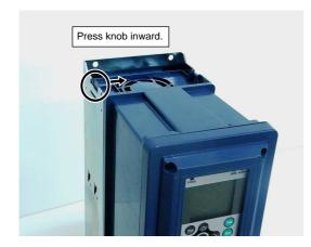
Remove the cooling fan (with case).
